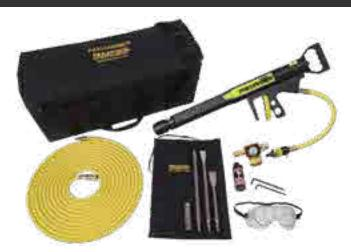
A 1000-1100 high impact blows per minute, 11 pound impact tool that dramatically increases the range of forcible entry and rescue work initial responding units can handle without calling up heavy equipment. The Pakhammer is the only pneumatic impact tool of its size that is designed to operate from portable air cylinders. It is an ideal tool for bus and train rescue, high rise work, collapse rescue or any situation that requires a powerful impact tool that operates from a limited air supply.
