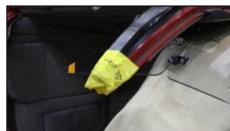
Cut or broken metal vehicle posts
