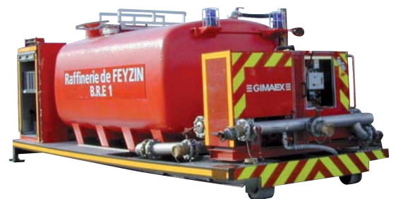
1000 l/min skid-mounted transfer pump with thermal engine
