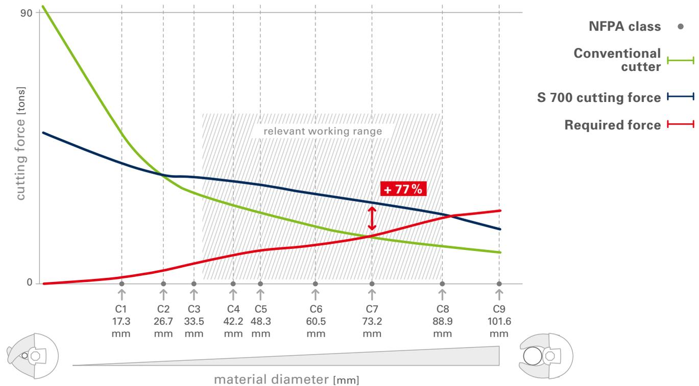
The car posts you need to cut are getting ever thicker and more stable. To ensure that you are optimally prepared, **LUKAS** no longer takes part in the race for theoretical maximum force. With the S 700, we have instead developed a cutter in which blade opening and force application are perfectly matched to the relevant working range.
