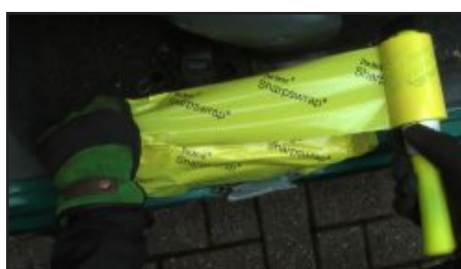
Dangerous projections or sharp metal edges in wrecked vehicles
