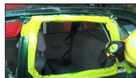
Window frames after glass is removed or broken
