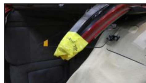
Cut or broken metal vehicle posts
