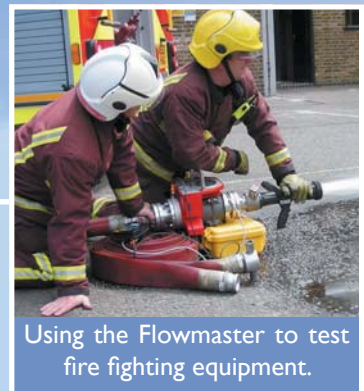
Using the Flowmaster to test a fire pump.
