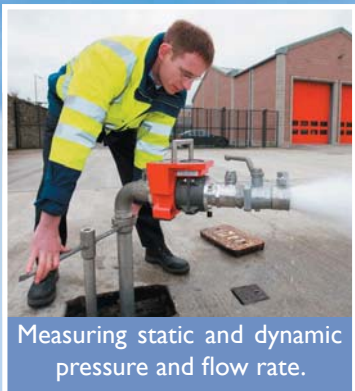
Using the Flowmaster to test a fire hydrant.
